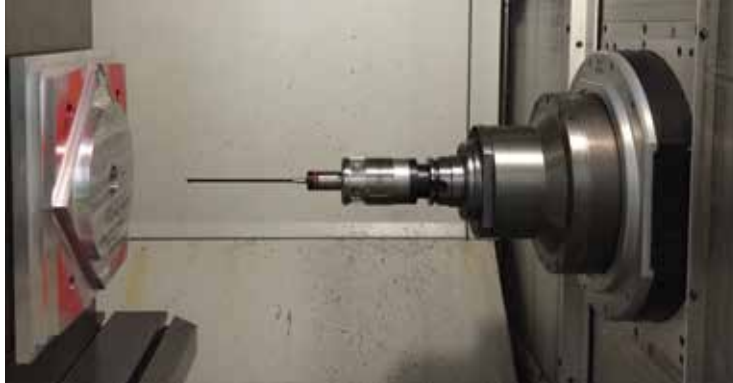
The Jakob motor spindle safety system, the MS 3 , is designed for vertical and horizontal machining centers.
